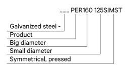
Sample: PER160125SIMST – made of galvanized steel, reducer from 160mm to 125mm, symmetrical, pressed.
